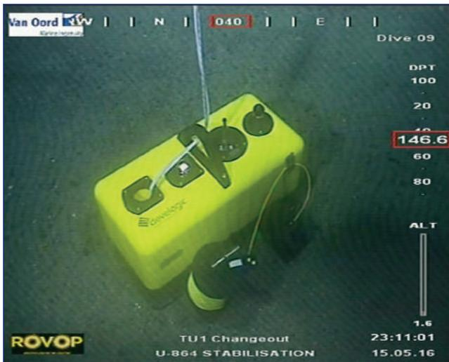
To meet these monitoring requirements, develogic delivered a turnkey monitoring system measuring sediment load and ocean current at several levels, as well as potential movement and vibration of the submarine hull due to the impact of the materials that make up the counterfill, together with deployment and operation support services.
