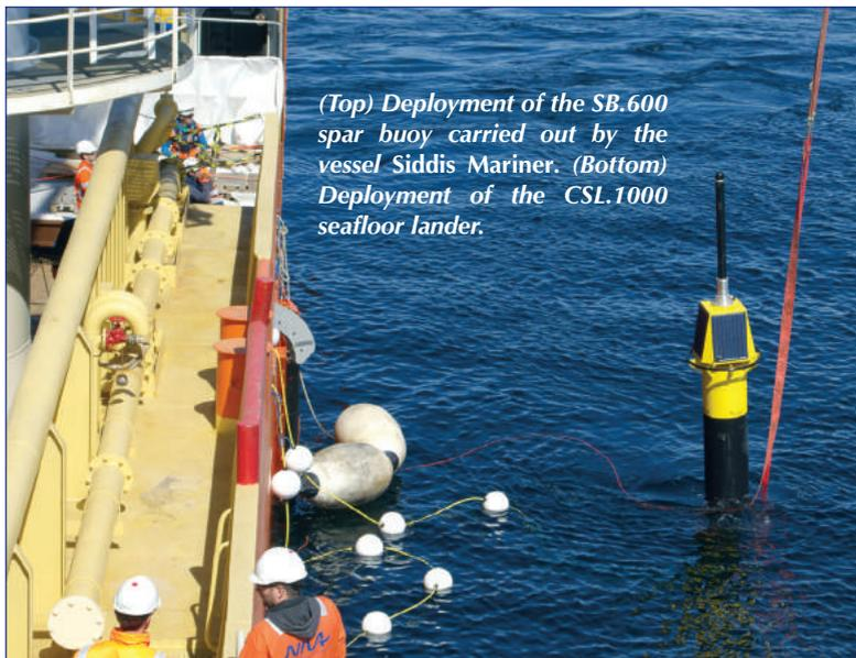
*(Top) Deployment of the SB.600 spar buoy carried out by the vessel Siddis Mariner. (Bottom) Deployment of the CSL.1000 seafloor lander.*
