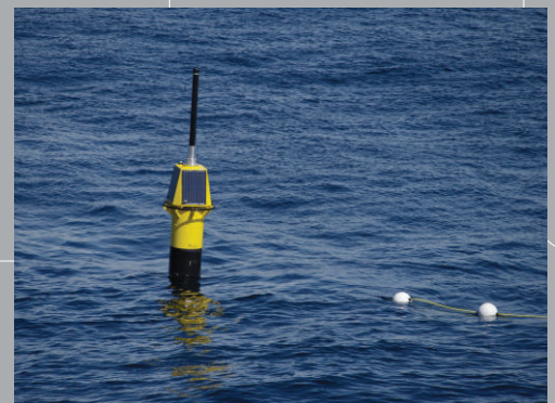
SB.600 spar buoy with inductive mooring (U864 counterfill operation)
