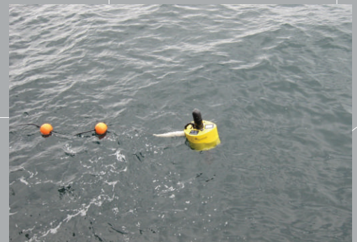
MI.Sat II buoy with inductive mooring
