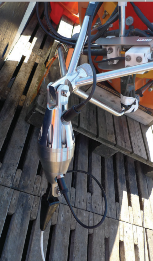
Swivel C.45 in inductive mooring (picture courtesy NOC)
